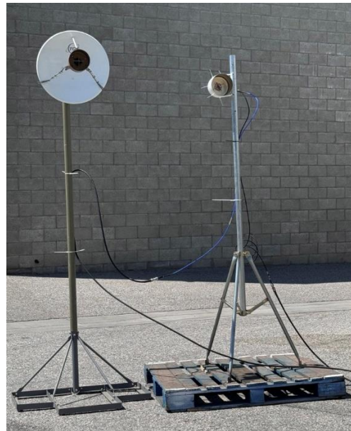
Figure 6 – Dipole in a cup boresight antennas
