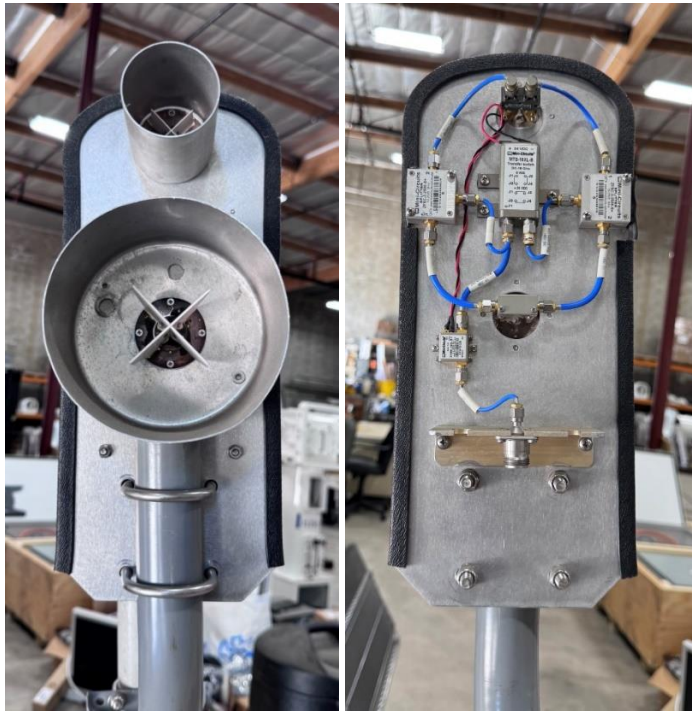
Figure 5 - Circularly polarized boresight antenna
