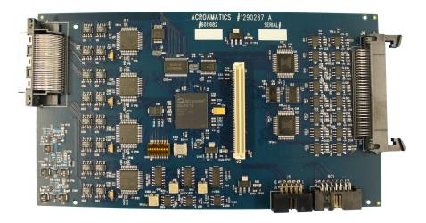
Model 682M is a mezzanine module for the PCle-bus Model 1635AP Programmable Data Stream Processor telemetry system EU processing and data distribution card.
