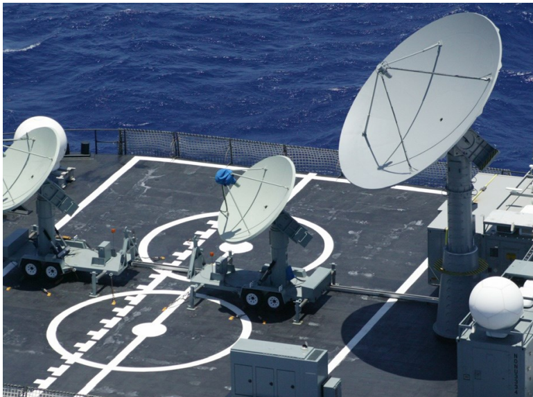
Here is a ship-stabilized, 7.3 meter Model 6000 System.
